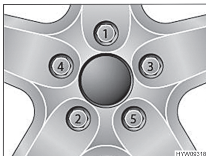
Fig. 90 Tightening the wheel nuts or wheel bolts cross-wise
