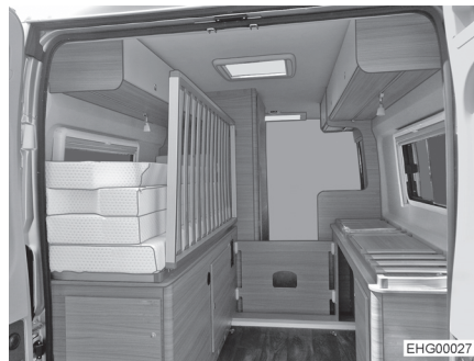
Fig. 35 Transport position (folding bed base)
