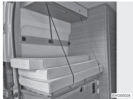
Fig. 36 Transport position (removable bed base)
